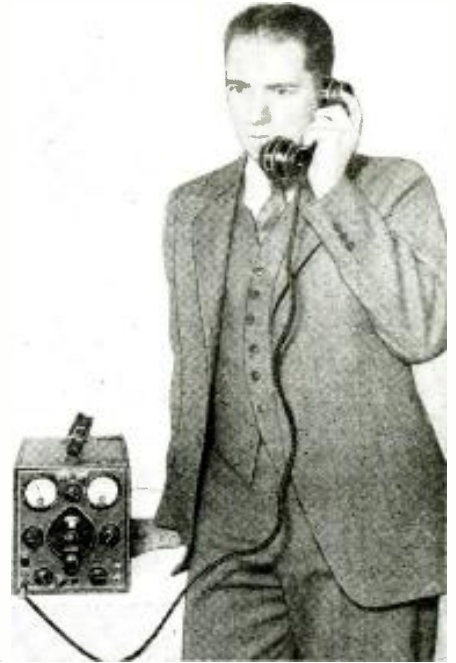
Here is the midget transmitter and receiver for 5-meter work with the author at the "mike."
