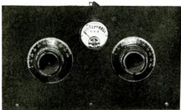
Front view of Mr. Shuart's latest simplified transmitter using the new 802 tube.
