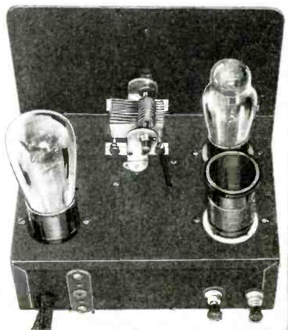
Top and bottom views of the excellent beginner's receiver, showing placement of the various parts.
