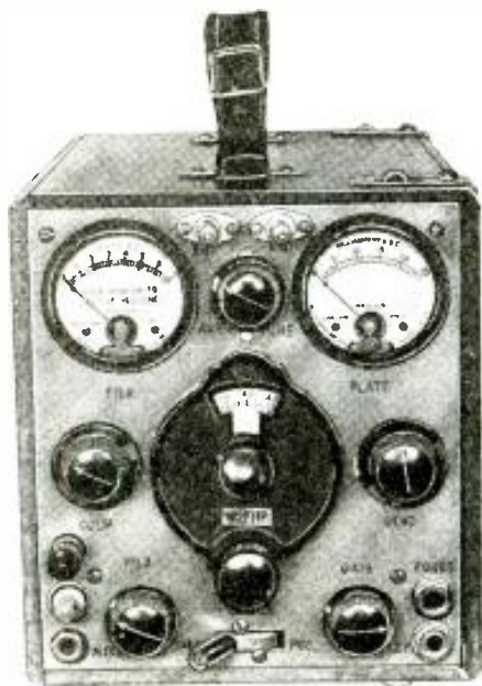
Front panel view of the De Luxe 5-meter Transmitter and Receiver which the author has designed for portable use.
